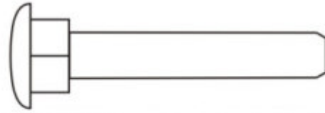
(40) M8X60mm Carriage Bolt 2pc
